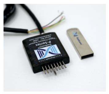
EvoScann® P-Series are highly-miniaturised pressure scanners designed specifically to meet the stringent demands of the aerodynamic testing industry where development is rapid and continuous. Utilising the latest in miniature scanner technology, P-Series is at the forefront of pressure measurement in challenging aerodynamic locations. P-Series has been designed, from the start, with physical size, weight, accuracy and functionality in-mind and is available in a variety of configurations.
