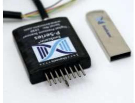
The EvoScann® P8D was developed to allow direct measurement of the dynamic pressures, whilst simultaneously, in real time, eliminating offsets caused by changes in barometric pressure; a True Differential pressure measurement device.
